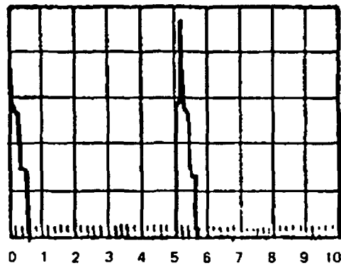
Figure 5.15 (b) : CRT screen display for 200 mm test range calibration (when the probe is positioned at 'E').
