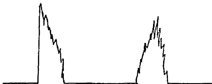
Figure 8.17 : Shape of echo from a slag inclusion.
