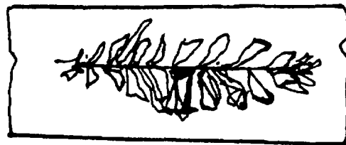
Figure 1.40 : Piping in weld.
