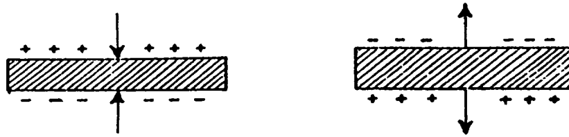
Figure 2.18 (a) : Direct piezoelectric effect.
