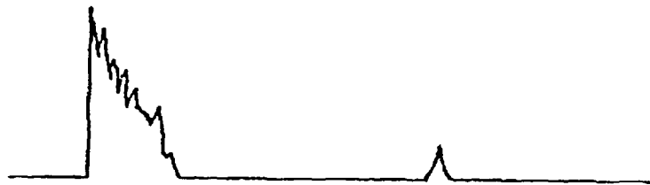
Figure 8.15 : Shape of the echo from a pore.
