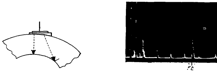
Figure 6.40 : Testing method for detecting longitudinal surface defects on internal surfaces of thick wall tubes using normal probes.
