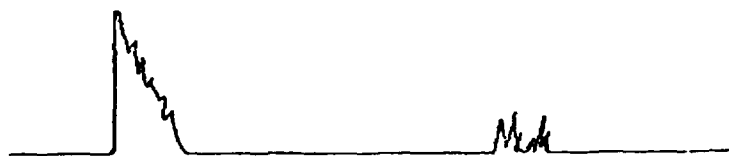
Figure 8.16 : Shape of echoes from porosity.
